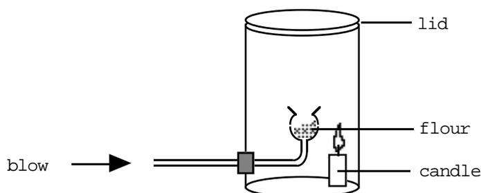
When the flour is blown out into the can, the candle sets it on fire. Because of the small particle size it burns very quickly and gives out a lot of energy. The lid of the can blows off!
