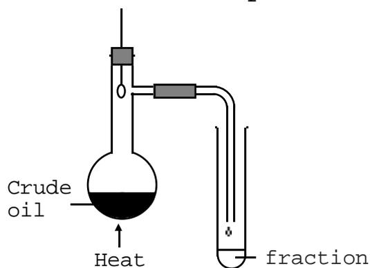
As the crude oil is heated, the compounds with the lowest boiling points begin to boil out of the mixture and condense in the test tube. Fractions can be obtained which contain groups of compounds with boiling points within a given range.
