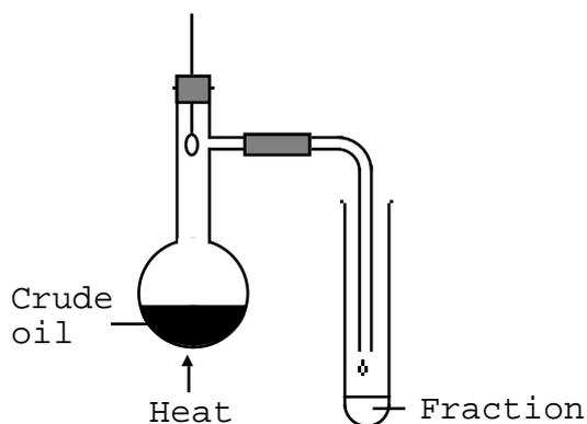
The oil is gradually heated. Fractions, groups of hydrocarbons with boiling points within a given range, are collected.
