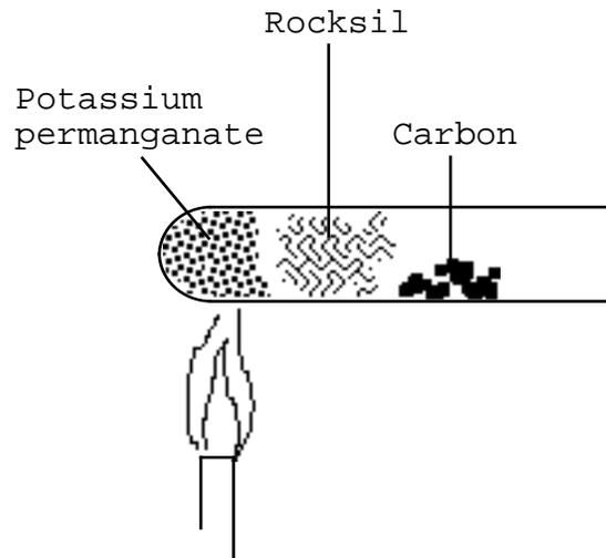
Potassium permanganate gives off Oxygen gas when heated. The Oxygen passes across the hot Carbon. The Carbon burns (orange to white-hot). Red hot sparks of burning Carbon are thrown out of the test-tube. Heat and light energy are produced.
