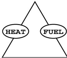
When a substance burns it reacts with Oxygen. Remove the Oxygen and the fuel cannot burn.
