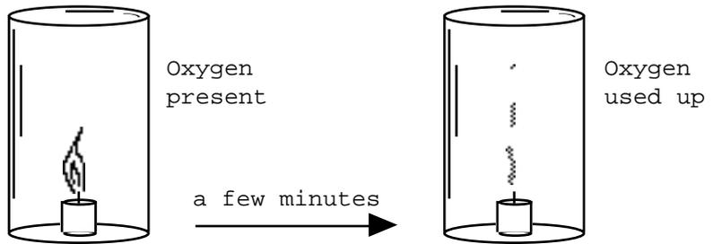
The burning candle reacts with the Oxygen inside the jar. When all the Oxygen is used up the flame goes out.
