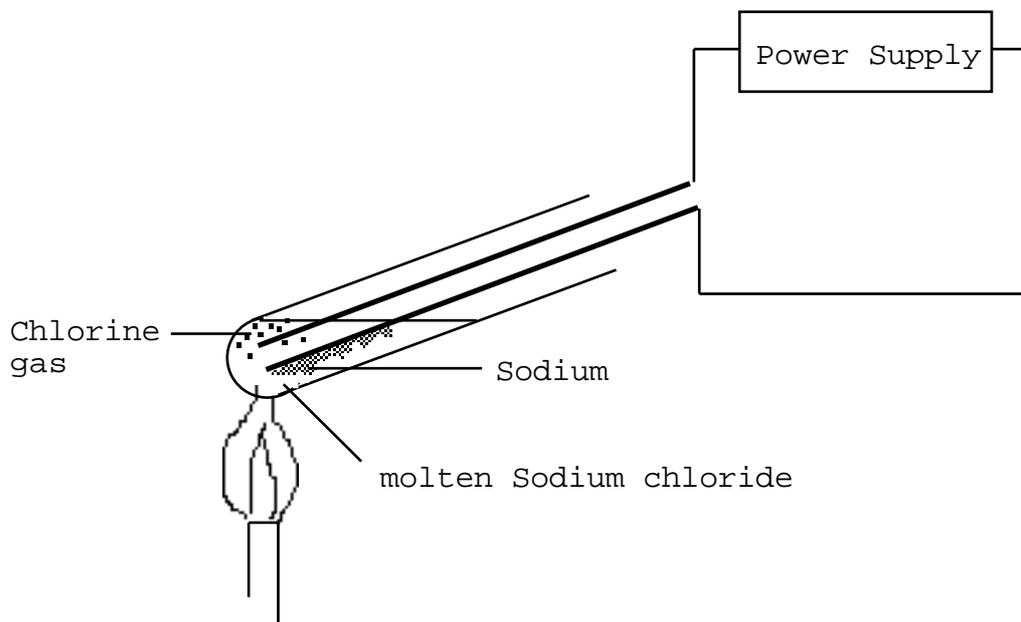
Sodium is obtained at one of the electrodes.
