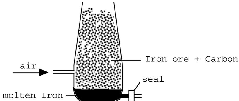
The mixture is heated. Air is forced in at the bottom. The air rushes up through the furnace making a roaring sound. Some of the Carbon burns in the Oxygen. The heat generated raises the temperature of the furnace and the reaction between Iron oxide and Carbon begins:
