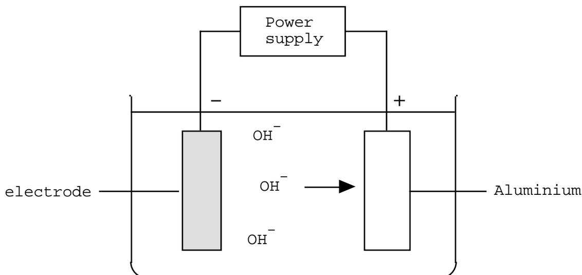
The piece of Aluminium forms the positive electrode. The negative ions are therefore attracted to the positively charged Aluminium and react with it forming Aluminium oxide.
