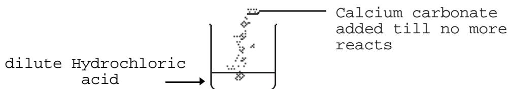
When the reaction is over (no more bubbles of Carbon dioxide) the excess Calcium carbonate can be filtered off since it is **not** soluble in Water. The Calcium chloride is obtained by evaporation of the filtrate.
