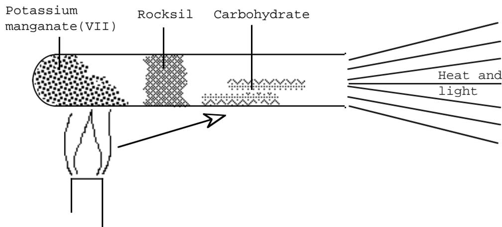
Heating Potassium manganate(VII) gives off Oxygen. The Oxygen passes across the hot carbohydrate which bursts into flames giving out heat and light energy.
