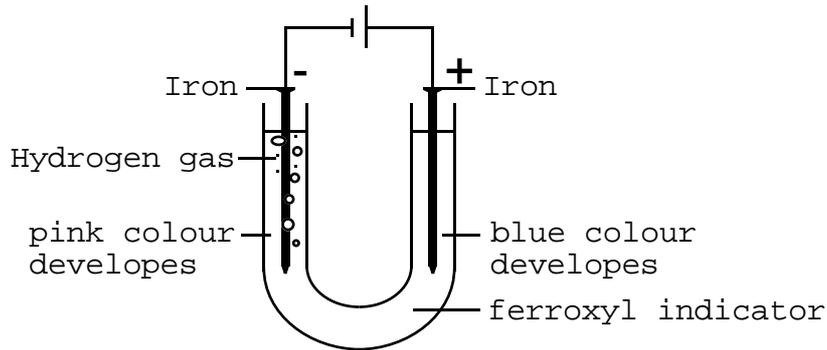
At the anode (+ve) electrons are pumped away from the Iron, speeding up the corrosion rate :
