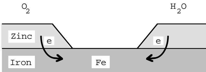
the Oxygen and Water can get to the Iron but corrosion still does not occur because electrons flow from Zinc to Iron preventing loss of electrons by Iron. Bridge girders are galvanised.
