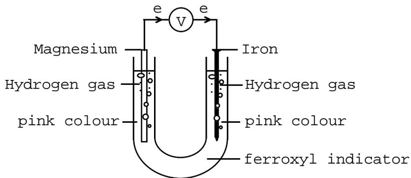
NO blue colour appears round the Iron so no Iron(II) ions are being produced.
