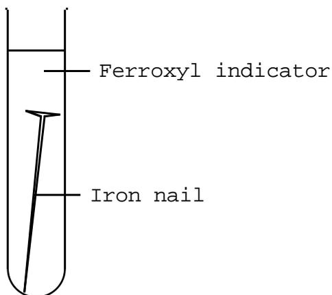
Ferroxyll indicator turns BLUE in the presence of  $\text{Fe}^{2+}$  ions. A BLUE colour appears round the Iron showing that  $\text{Fe}^{2+}$  are formed.
