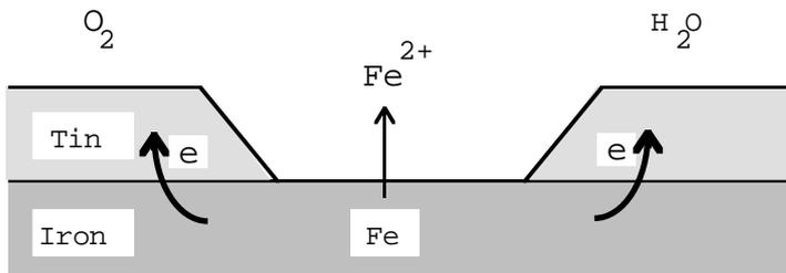
Corrosion is more rapid than in an uncoated piece of Iron : the Tin(II) ions pull electrons off the Iron :
