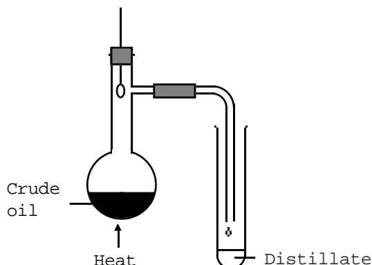
The oil is gradually heated. The small gas molecules boil off first, at low temperatures. We call this the 'gas fraction'. It consists of  $\text{C}_1$  to  $\text{C}_4$  hydrocarbons e.g. Butane  $\text{C}_4\text{H}_{10}$  (BP  $0^\circ\text{C}$ ). The gas fraction is used to make Calor Gas.
