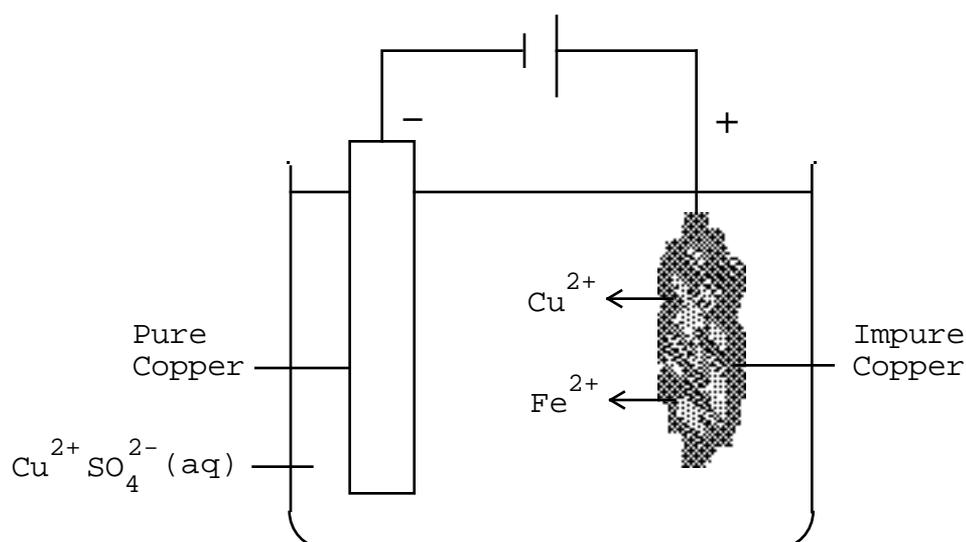
The anode draws electrons away from Cu and Fe.
