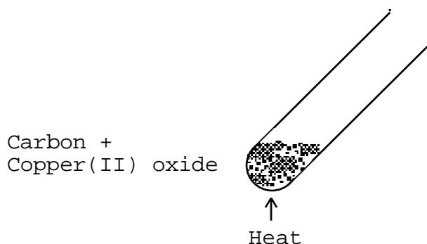
Carbon monoxide is produced by reaction of Carbon with Oxygen in the air. The Carbon monoxide then reacts with the Copper(II) oxide :
