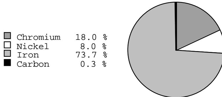
The properties of an alloy vary with its composition e.g. the more Carbon in steel the harder it becomes.
