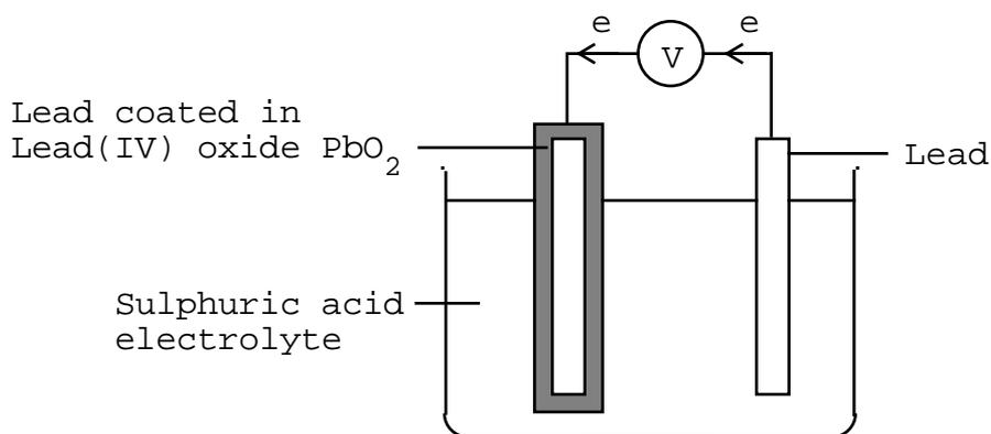
Electrons flow from Lead to Lead(IV) oxide ( $V = 2.03$  volts)
