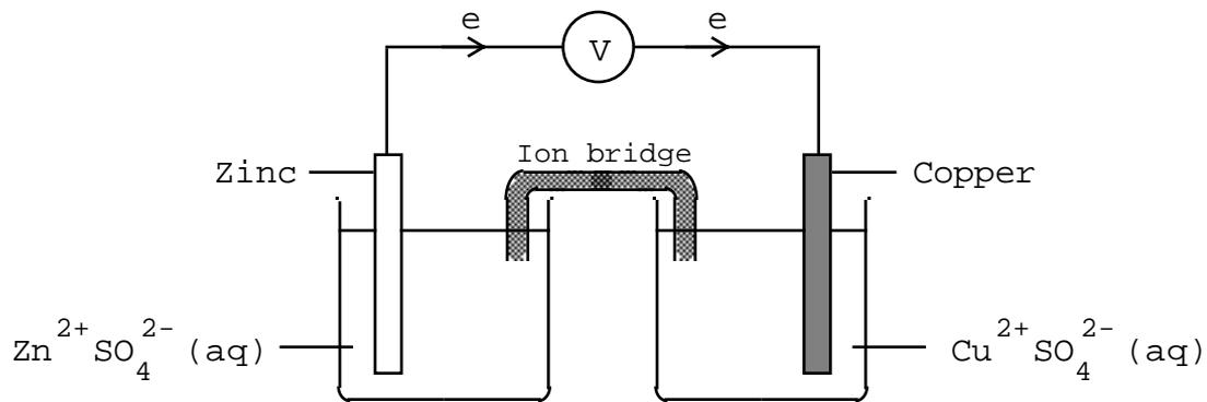
Electrons flow from Zn to  $\text{Cu}^{2+}$  along the wires and through the voltmeter. This is an electric current ( $V = 1.10 \text{ V}$ ).
