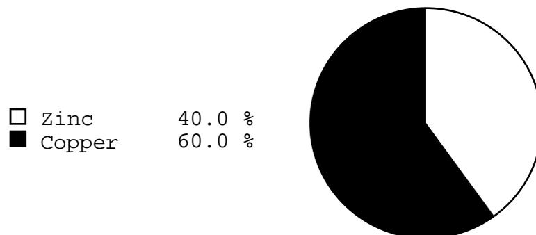
Brass is stronger than either Copper or Zinc and does not corrode. It is used to make shell cases, electric plugs etc.
