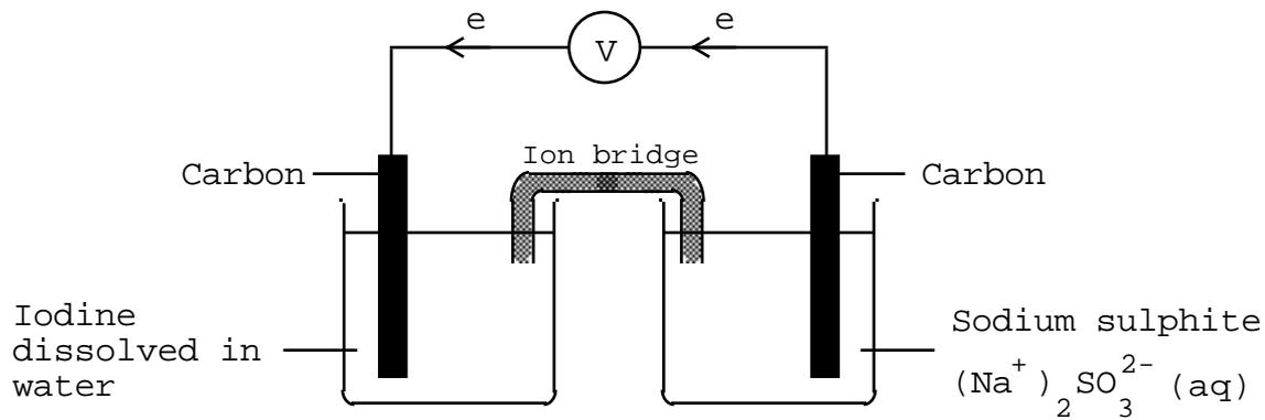
Electrons flow from Sodium sulphite to Iodine ( $V = 0.37$  volts) :
