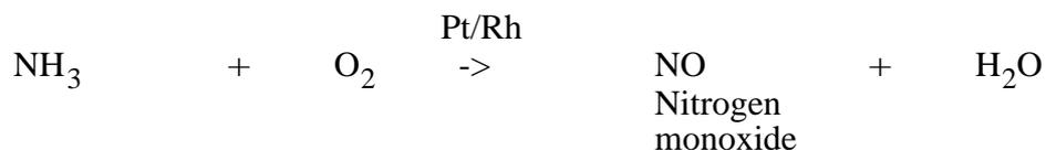
High temperatures must be used to increase the violence of the collisions between  $\text{NH}_3$  and  $\text{O}_2$  so that bonds will break and new bonds form. The catalyst is in the form of a sheet of gauze. Electricity is passed through the gauze to heat it. The reaction is exothermic (gives out heat). Once the reaction has started, the heat given out heats up the catalyst and so the electrical heating can be turned off.
