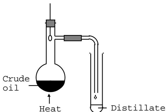
The fractions boil off in the order : gases, petrol etc.
