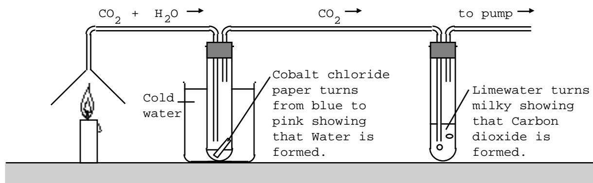
Notice that this experiment shows that hydrocarbons must contain Hydrogen : the Hydrogen in the Water formed can only have come from the hydrocarbon. Similarly the experiment shows that hydrocarbons must contain Carbon : the Carbon in the Carbon dioxide can only have come from the hydrocarbon.
