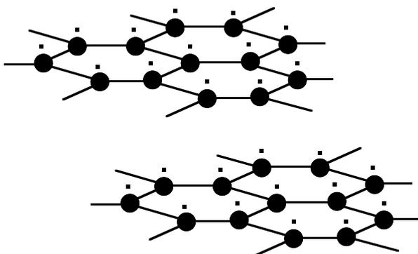
Graphite conducts (remember Carbon electrodes!) because each Carbon atom has one unpaired electron not used in bonding. These unpaired electrons 'swarm' across the layers and are responsible for the current.
